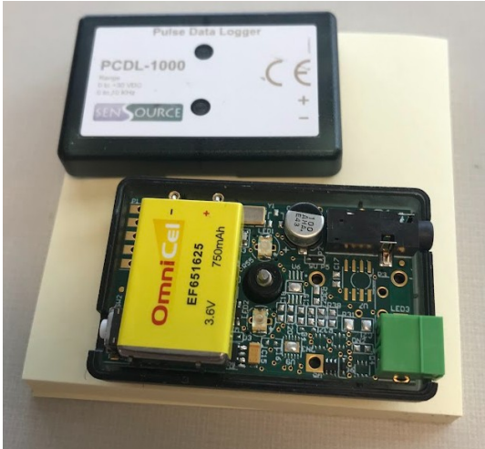
Failed "Pulse Data Logger" hardware
