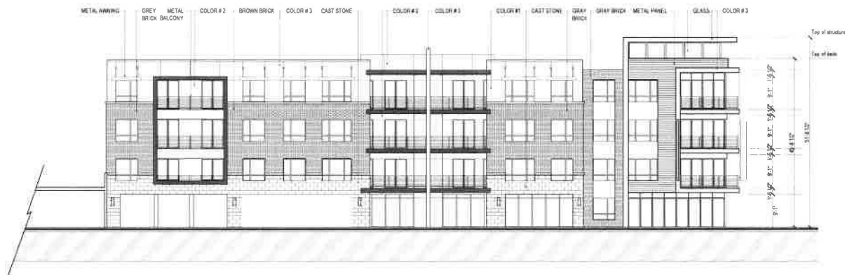
SIDE ELEVATION ( South/ pool courtyard)
