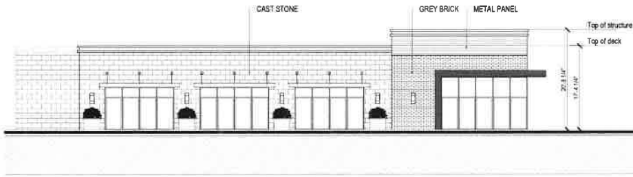
SIDE ELEVATION BRICK 17% CAST STONE 74% METAL PANEL 9%
