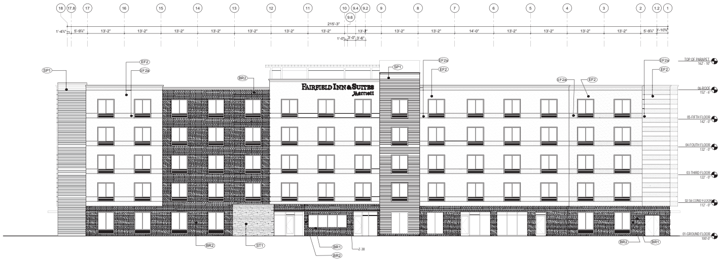
2 EXTERIOR ELEVATION - NORTH 3/32" = 1'-0"
