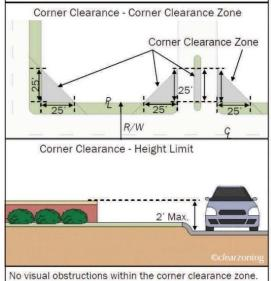
Obstructions to vision above a height of 2', measured from established street grade, are not allowed. Plant
