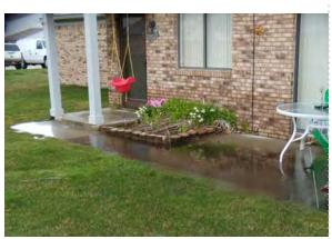
SDA performed a field investigation during a rain event and evaluated site grading and condition and function of the storm drainage system. SDA obtained record documents to compare actual site conditions to the original proposed design to assist with preparing final recommendations. SDA prepared a final report with findings identifying deficiencies in the drainage system and final recommendations with associated cost estimate.
