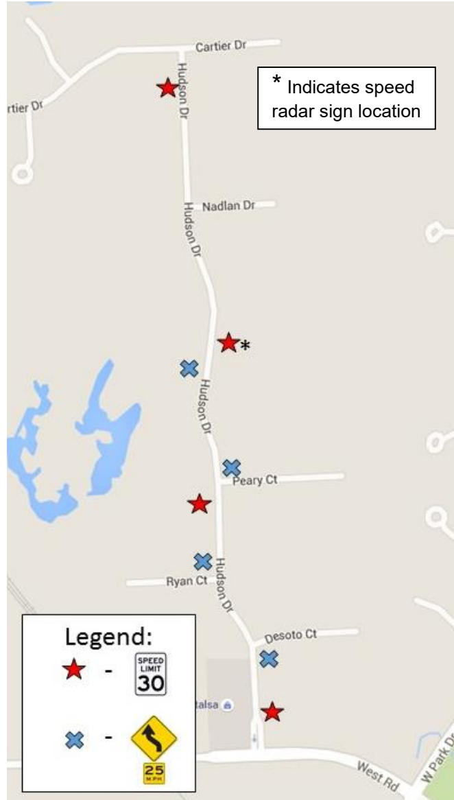
Figure 4: Proposed regulatory and warning signing locations along Hudson Drive (not to scale)
