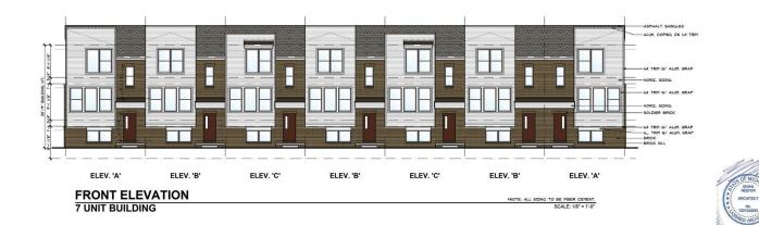
FRONT ELEVATION MATERIAL ALLOWABLE PROPOSED PERCENTAGE BRICK 100% 1,083 SF 33% 1,296 SF 39.5% SIDING 0% SHINGLES 25% 454 SF 14% TRIM 15% 444 SF 13.5% TOTAL 3,211 SF 100%
