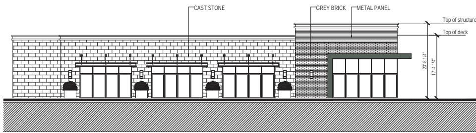
SIDE ELEVATION BRICK 17% CAST STONE 74% METAL PANEL 9%
