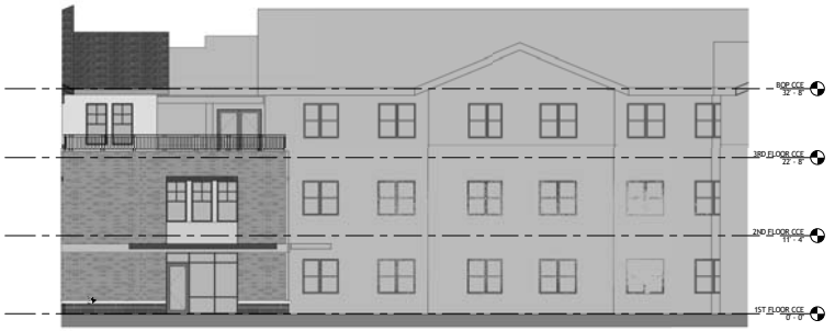
3 SOUTH ELEVATION COURTYARD (A4.10) (A4.20) 1/8" = 1'-0"
