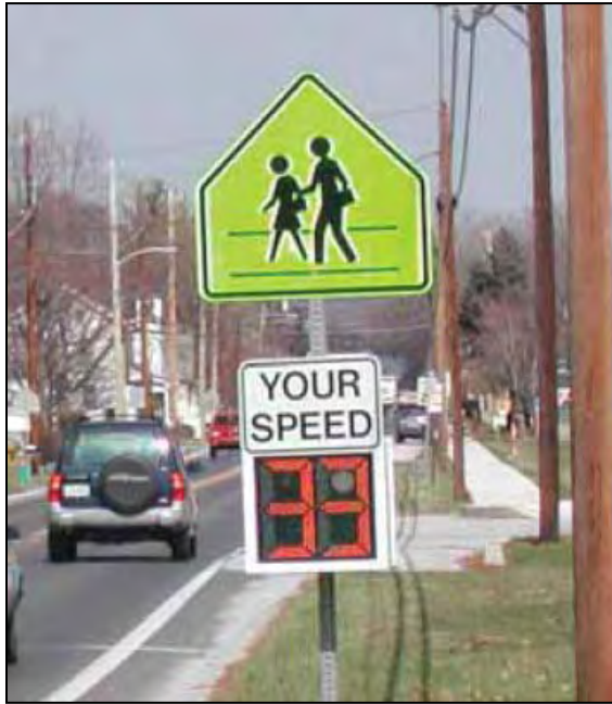
Fig. 5.7F. Portable Speed and Traffic Detectors
