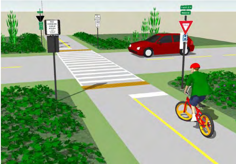
Fig. 5.11C. Trail Signs at Road Intersections Trail View
