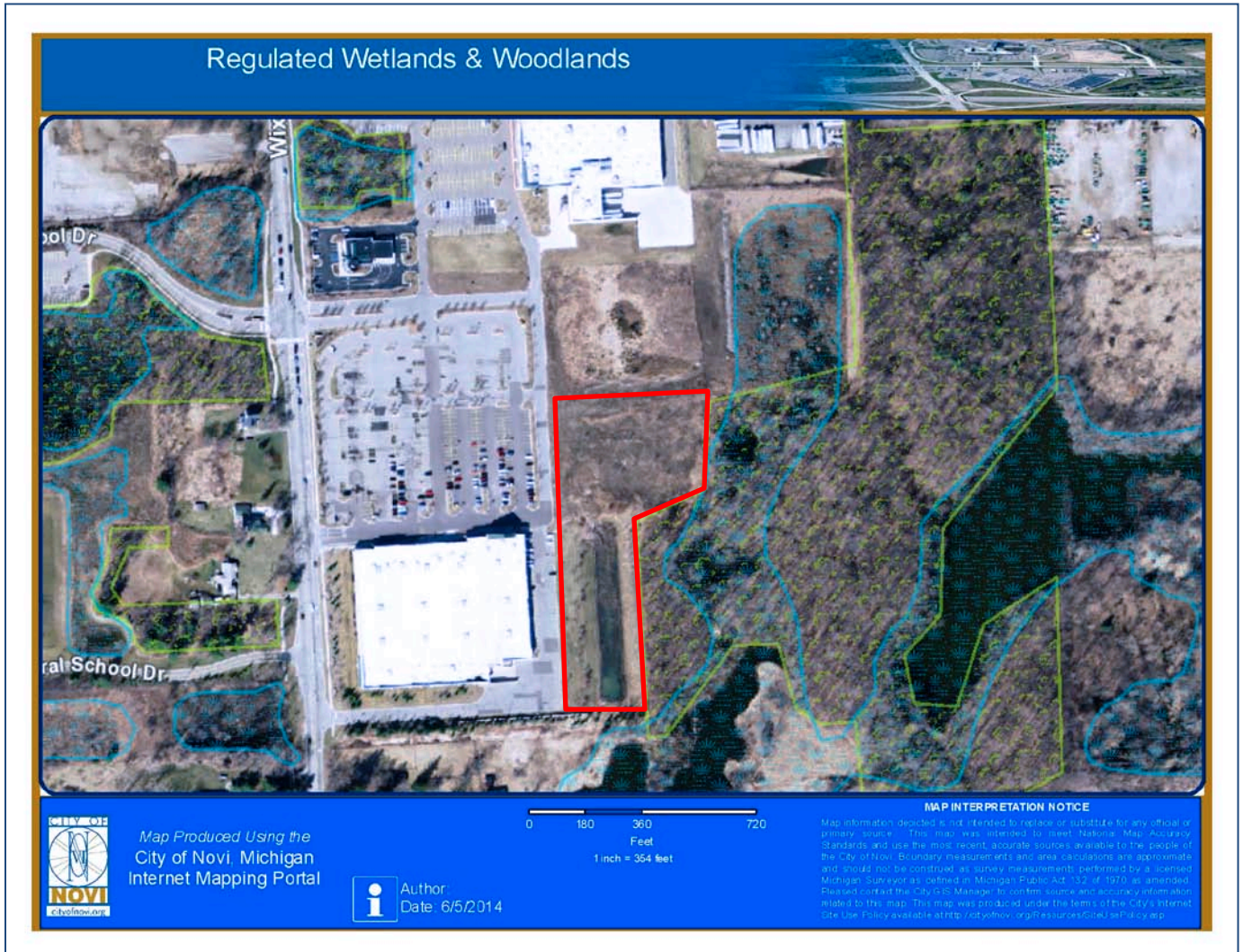
Figure 1. City of Novi Regulated Wetland and Woodland Map (accessed June 5, 2014). Regulated wetland boundaries are shown in blue. The approximate project boundary is shown in red.
