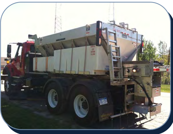
Plow Truck Equipped with Brine Tanks and Pre-Wet System
