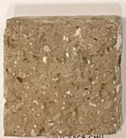
SPLIT FACE CMU
