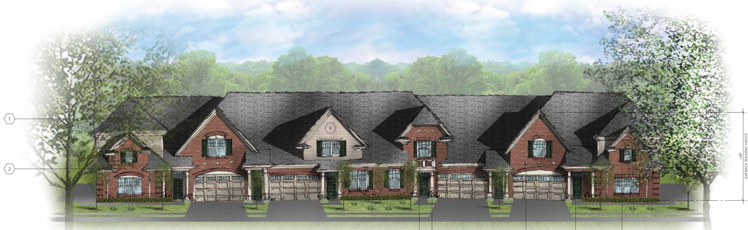
BUILDING 100 (10 UNITS) - FRONT ELEVATION 'C' (2) THREE BEDROOM UNITS SCALE: 1/8" = 1'-0" NOTE: BUILDING 150 (5 UNITS) SIMILAR
