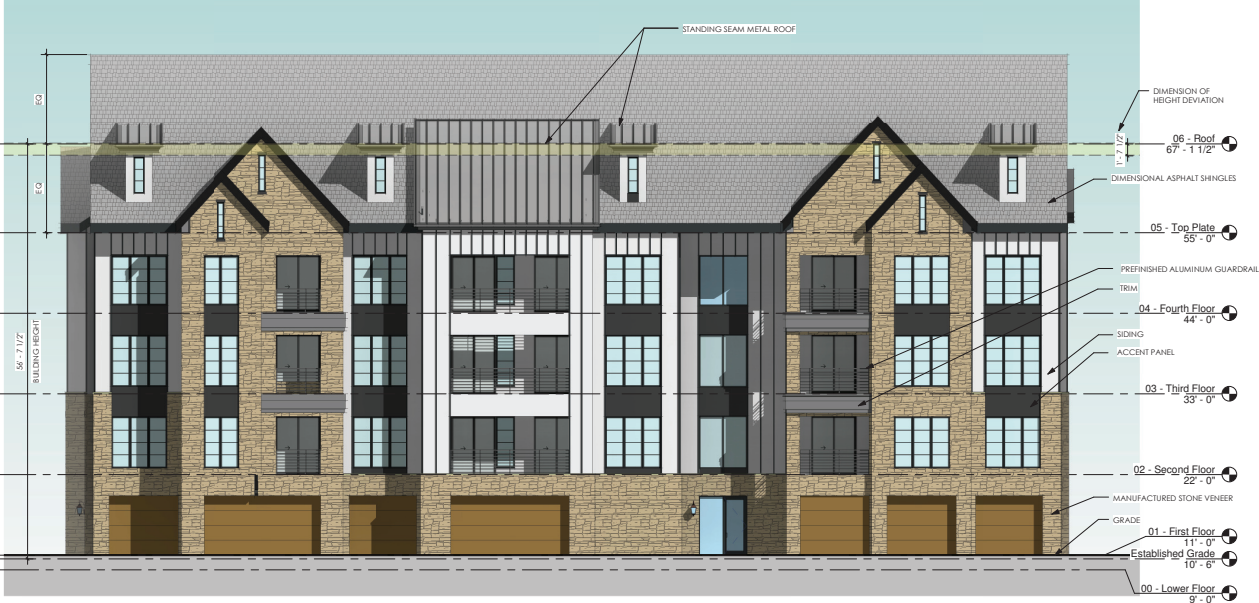
c Northeast Elevation A.106 1/8" = 1'-0"
