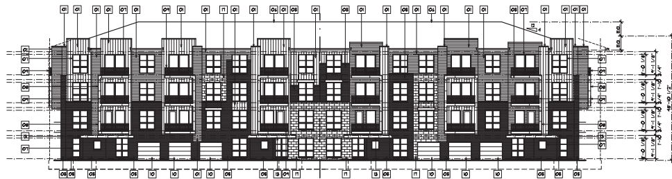
REAR ELEVATION BUILDING 255 BUILDINGS WILL STEP TO FOLLOW FINAL GRADE - SEE CIVIL DRAWINGS SCALE: 1/16" = 1'-0"
