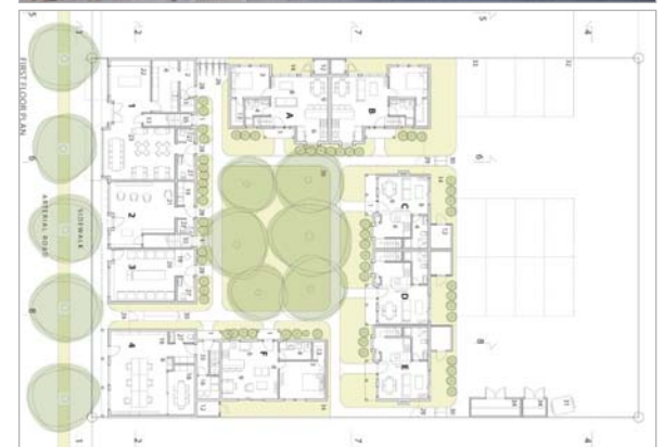
Images above: This courtyard development with adjacent live-work units designed by Niko Tiula won Opticos Design's Michigan Missing Middle Housing design competition in 2015. It offers higher density and mixed use at a modest scale.
