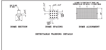
DETECTABLE WARNING DETAILS
