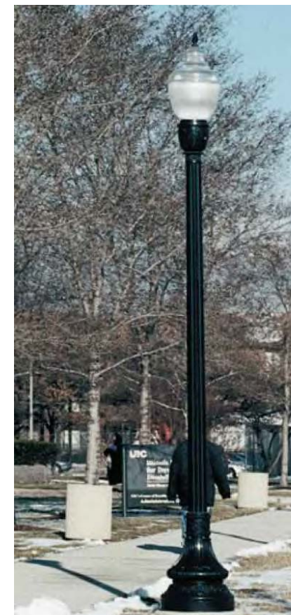
4G decorative light and pole (1-CONDITIONS) DECORATIVE POLE AND STREET LIGHTS MANUFACTURED BY HALOPANE LIGHT FIXTURE: WASHINGTON SERIES-ACRYLIC MODEL NO. AW100HF12B5DNB OR EQUAL POLE: WADSWORTH SERIES MODEL NO. AW100HF12B5DNB OR EQUAL POLE HIGH: 12' HIGH FINISH: BLACK POLE DIAMETER: 5" POLE BASE: 12"
