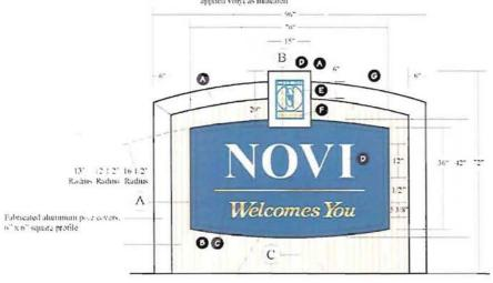
Fabricated alumnum sign cabinet, beveled edges. Cut-out aluminum text and rule line to be mechanically attached to sign face.
