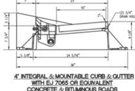
4' INTEGRAL & MOUNTABLE CURB & GUTTER WITH EJ 7065 OR EQUIVALENT CONCRETE & BITUMINOUS ROADS DETAIL - 3b NOT TO SCALE
