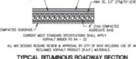
TYPICAL BITUMINOUS ROADWAY SECTION FOR RESIDENTIAL ROAD DETAIL - 1b NOT TO SCALE
